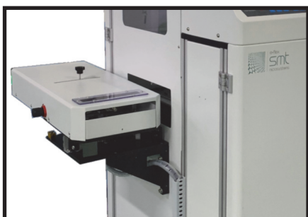
Status when the pusher box is folded
