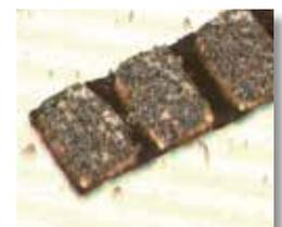
2D+3D Image with clear low bridge defect
