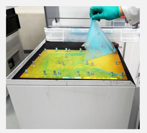
If sealed coating carriers or chamber elements are as heavily contaminated by varnish residues that optimal function is no longer guaranteed, these residues can be quickly removed by simply peeling off the CarrierSeal® sealing.
