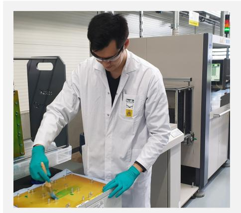
With a brush with synthetic bristles the slightly pasty CarrierSeal<sup>®</sup> liquid is distributed evenly and comprehensively on the carrier and its mounted build-ups.
