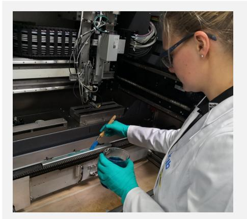
Or distribute **kolb** CarrierSeal<sup>®</sup> in the same way on the areas / machine parts that you want to seal.
